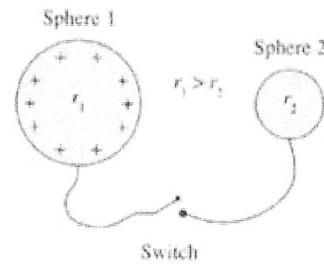
*Equal. When switch close, sphere 1 + sphere 2 + wire act as a single conductor. In equil. the potential of a conductor is everywhere the same.*
