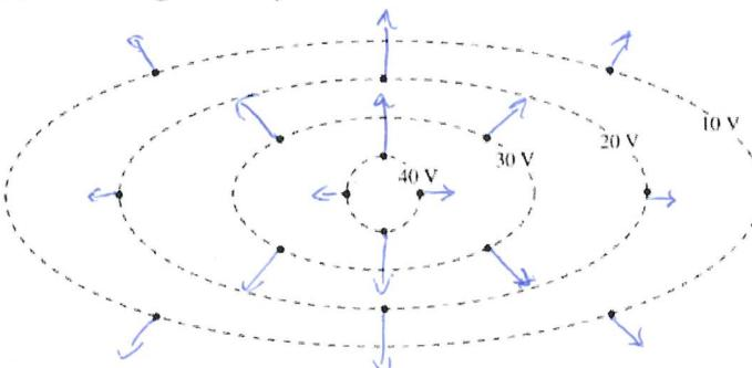
Draw the electric field vectors at the dots on this contour map. The length of each vector should be proportional to the field strength at that point.
